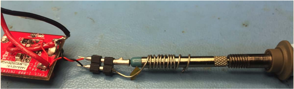
FIGURE 14. CONNECTION USING NEW HIGH FREQUENCY INTERCONNECT METHOD
